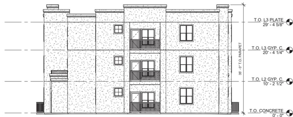
② LEFT ELEVATION - BLDG. TYPE A
