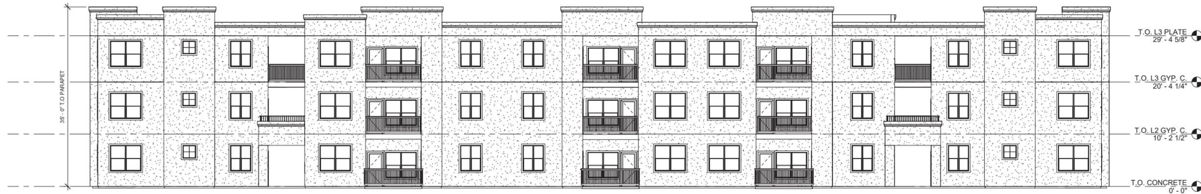
① FRONT ELEVATION - BLDG. TYPE A
